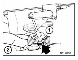
Remove retaining bracket (1) of angle joint from control arm (2).
