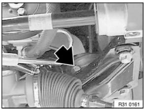
Remove control arm bracket from engine support.
